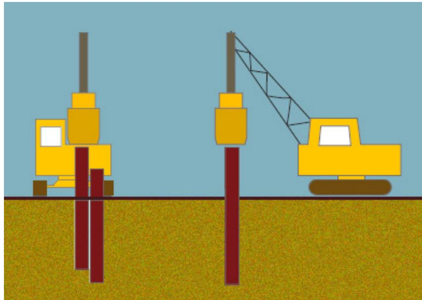
The piling rig lifts a first sheet pile and drives it into the ground. The same cycle is repeated for the next sheet pile and drives it into the ground as it interlocks with the previous sheet pile. There is no interlocking between H beam driven piles. The space between the sheets is filled with filler members.
